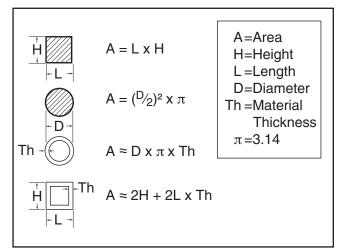
Figure 21. Calculating cut area for break-in.
